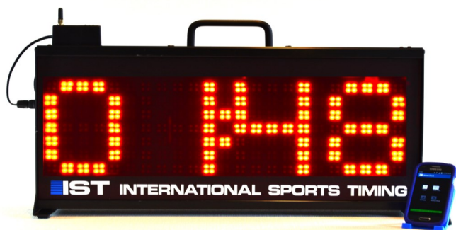
SWIMCOUNT shown with Bluetooth adapter and Android Smartphone
